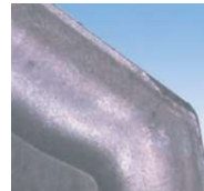
Abrasion on rake face
